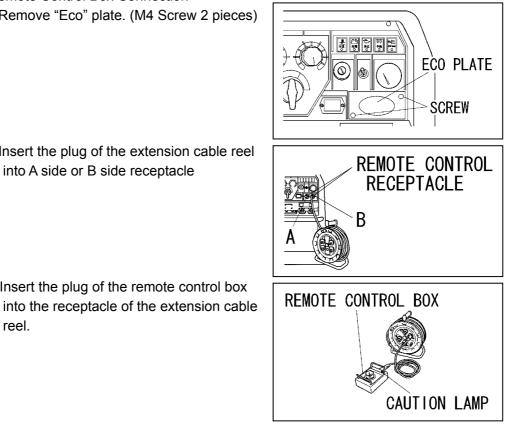
Insert the plug of the extension cable reel into A side or B side receptacle
